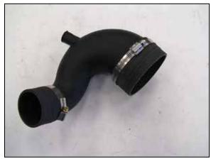
15. Install the provided coupler hoses (5-222N and 08761) onto the Passenger side intake tube (9-0461) and secure with the provided hose clamps.
