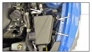
6. Remove the three bolts that secure the driver side air filter housing to the inner fender, loosen the hose clamp that secures the intake tube to the air filter housing and disconnect the tube. Remove the driver side air housing from the vehicle.
