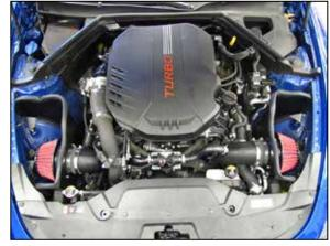
20. Install the provided AEM® air filters onto the filter adapters and secure with the provided hose clamps.
