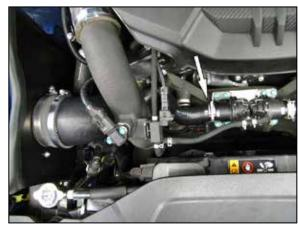
19. Install the driver's side BOV hose and secure with the factory hose clamps.
