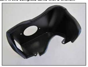
11. Trim and install the edge trim 35", 16" and 2-1/2" onto the driver's side heat shield (20-8633) as shown.
