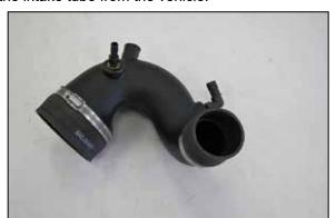
10. Install the provided couplers (5-222N & 08761) onto the Drivers side intake tube (9-0459) and then install the 90° and straight vent fittings as shown. NOTE: Plastic NPT fittings are easy to cross thread. Install the vent fitting "hand" tight, then turn it two complete turns with a wrench.
