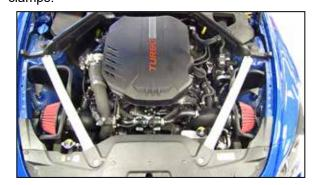
21. Reinstall both strut tower braces and secure with the factory hardware.
