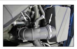
5. Loosen the hose clamps that secure the intake tube to the air filter housing and turbo inlet and then remove the intake tube from the vehicle.
