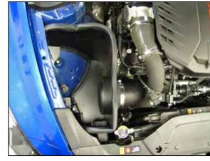
18. Install the provided filter adapter into the heat shield so that it goes through the heat shield and into the coupler on the intake tube. Secure the adapter to the heat shield using the provided hardware and then adjust the intake tube and couplers for best fit and secure with the provided hose clamps.
