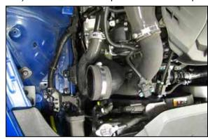
16. Install the passenger side intake tube onto the turbo inlet.
